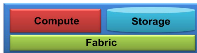
Figure 1: Windows Azure has three main parts: The Compute service, the Storage service, and the Fabric upon which both depend.
